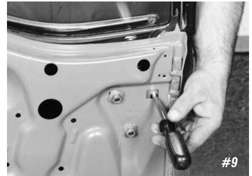
Photo #9: Using a large Phillips screwdriver, align the hole in the quarter base with the hole in the pivot assembly; and then install the special bolt, flat washer, and lockwasher. (See Photo #9) Do not tighten this bolt at this time.
